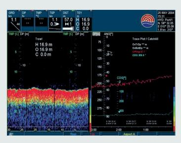
TrawlEye and GridSensor used on a small shrimp trailer. Shrimp influx can clearly be seen on the left side of the screen, which shows the TrawlEye.
